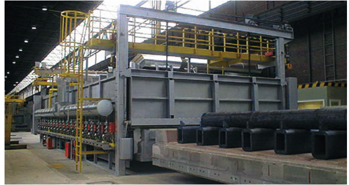
Metallurgical industry: bogie hearth furnace
