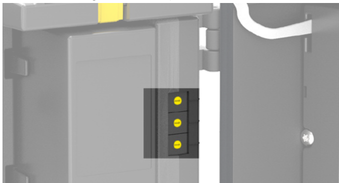
Code switch setting: upper switch (S1) = 10^2 (hundreds), centre switch (S2) = 10^1 (tens), lower switch (S3) = 10^0 (ones)
