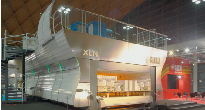
Roller hearth furnace
