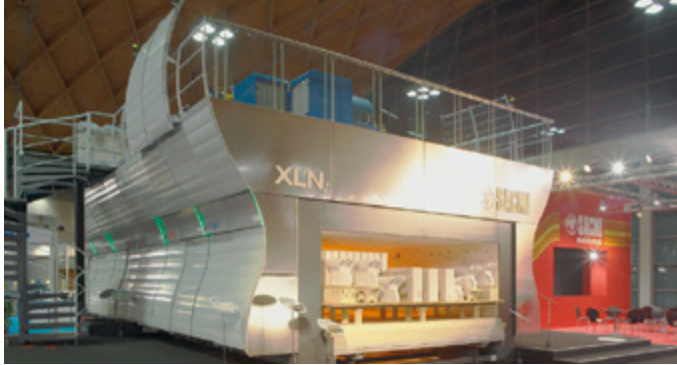
Roller hearth furnace
