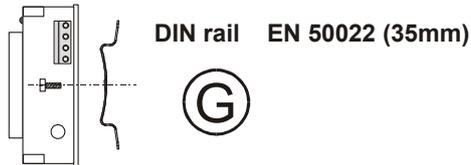
**!** G: Using the spring supplied, the CoCo-PC can be mounted on top hat rails
