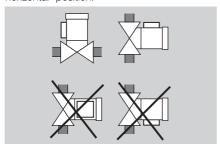
The motorized valve for gas VK must not be in contact with masonry. Minimum clearance 20 mm.
