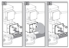
4 If there is oil on the upper housing cover (more than a few drops), remove the motor actuator and send it to the manufacturer.
