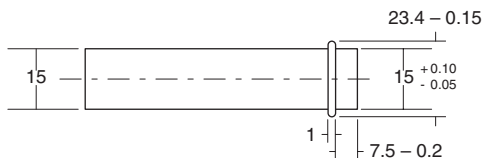
Fig. 18. Pipe end for "O"-ring connection for G 3/4" external thread
