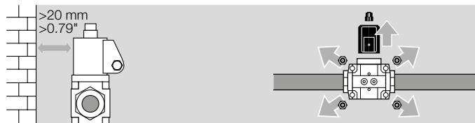
The magnetic relief valve VAN must not be in contact with masonry. Minimum clearance 20 mm (0.79 inches).
