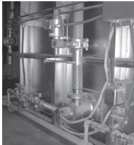
Chamber furnace in the refractory industry heated with excess air burners BIC 140LB.
